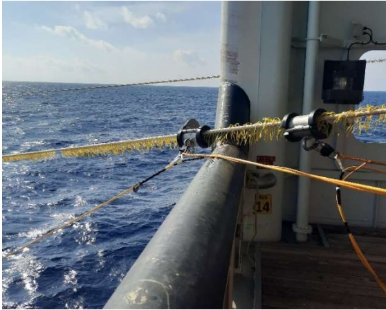
Figure 9. Slide collar over the lead-in (during deployment).
