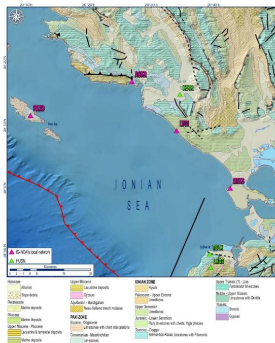
Figure 19 Geological map (IGME, 1983) of the portable (purple triangles) and permanent - HUSN (green triangles) seismographic station locations. The hatched yellow polygon represents the study area.
