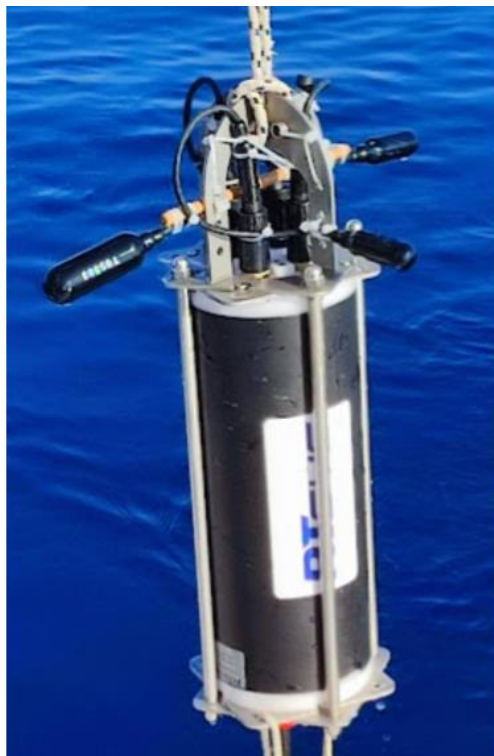
Fig. 2.1.2.1. The RT-SYS portable unit which used for measuring the ambient noise.
