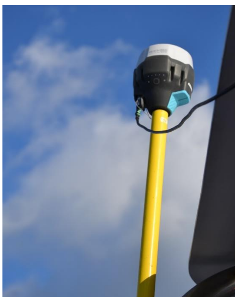
Fig. 2.1.2.3. The EMLID Reach GPS.
