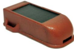
Figure 3-12. GPS-GSM device used for Scopoli's Shearwater telemetry
