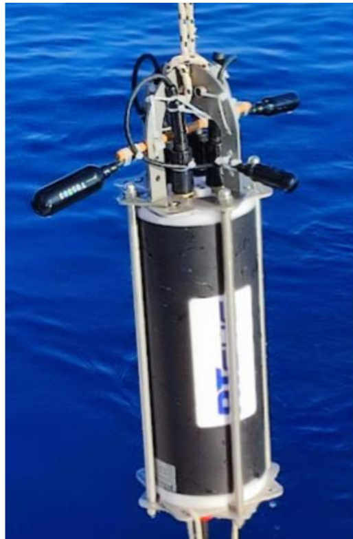
Fig. 2.1.2.1. The RT-SYS portable unit which used for measuring the ambient noise.
