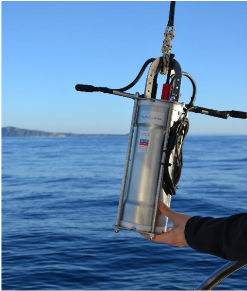
Fig. 2.1.2.1. The RT-SYS portable unit which used for measuring the ambient noise.
